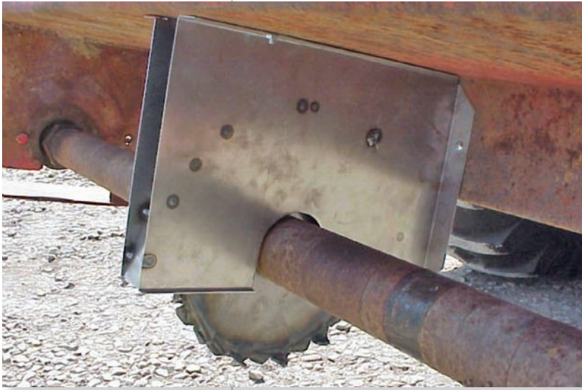
One of four rotating tiller blades mounted on a modified seeder and used to create the 2-inch-wide strip-seeded rows in perennial ryegrass plots and evaluate conversion to seeded Riviera bermudagrass. Photos by J. Fry
