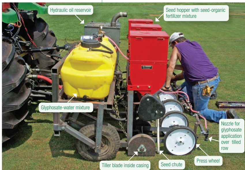
The strip-seeder was used to convert a perennial ryegrass turf to seeded Riviera bermudagrass.
