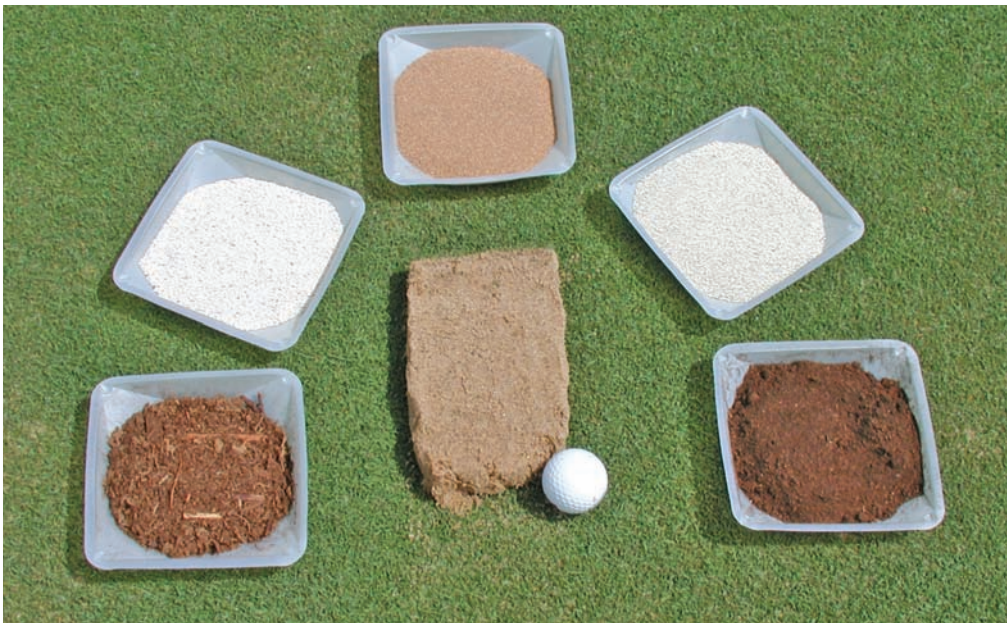
The root-zone amendments used in this research are (from left to right): sphagnum peat, zeolite, calcined clay, diatomaceous earth and reed sedge peat. Photos by D. Karcher
