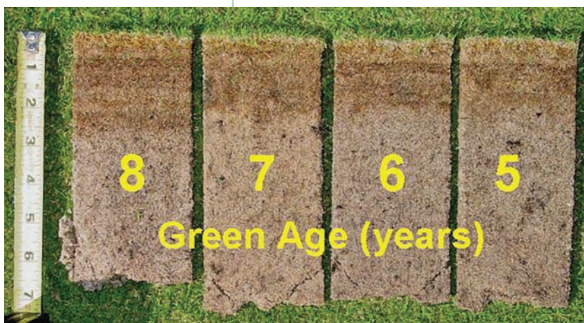
Figure 2. Profiles were collected from USGA 80:20 (sand:peat) greens on June 15, 2004. The profiles are from four greens aged five, six, seven and eight years. Photo by R. Gaussoin
