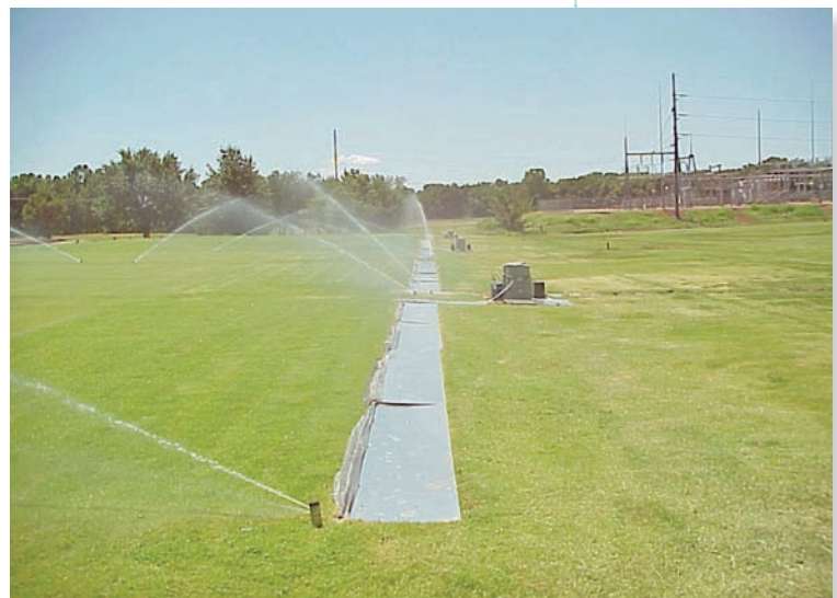
Covered troughs collected the runoff and channeled it through Parshall flumes by gravity flow.
