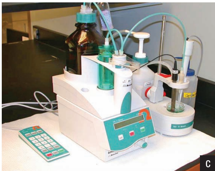
A diffusion unit was used to measure soil amino nitrogen content. (A) One gram of soil or a 0.2-gram sample of thatch was added to a Mason jar with sodium hydroxide. A petri dish containing 5 milliliters of boric acid indicator solution was suspended from the jar lid. (B) The sealed unit was placed on a hot plate at 118 F-122 F (48 C-50 C) for 5 hours. (C) After heating, the petri dish was removed, 5 milliliters of distilled water was added, and the solution is titrated with sulfuric acid. Amino nitrogen content is calculated as S \times 7 = amino nitrogen ppm, where S is the volume of sulfuric acid and T is the titer. Photos by D. Gardner
