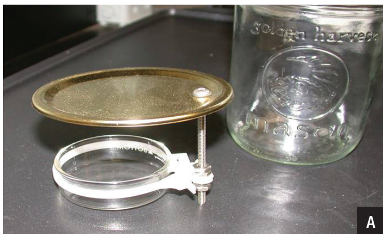
A diffusion unit was used to measure soil amino nitrogen content. (A) One gram of soil or a 0.2-gram sample of thatch was added to a Mason jar with sodium hydroxide. A petri dish containing 5 milliliters of boric acid indicator solution was suspended from the jar lid. (B) The sealed unit was placed on a hot plate at 118 F-122 F (48 C-50 C) for 5 hours. (C) After heating, the petri dish was removed, 5 milliliters of distilled water was added, and the solution is titrated with sulfuric acid. Amino nitrogen content is calculated as S \times 7 = amino nitrogen ppm, where S is the volume of sulfuric acid and T is the titer. Photos by D. Gardner
