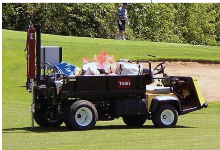
A hydraulic probe was used to collect soil cores from fairways in 2003 and 2004. Photo by B. Horgan
