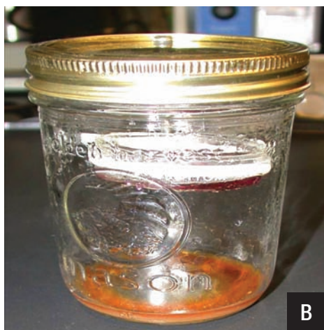
A diffusion unit was used to measure soil amino nitrogen content. (A) One gram of soil or a 0.2-gram sample of thatch was added to a Mason jar with sodium hydroxide. A petri dish containing 5 milliliters of boric acid indicator solution was suspended from the jar lid. (B) The sealed unit was placed on a hot plate at 118 F-122 F (48 C-50 C) for 5 hours. (C) After heating, the petri dish was removed, 5 milliliters of distilled water was added, and the solution is titrated with sulfuric acid. Amino nitrogen content is calculated as S \times 7 = amino nitrogen ppm, where S is the volume of sulfuric acid and T is the titer. Photos by D. Gardner
