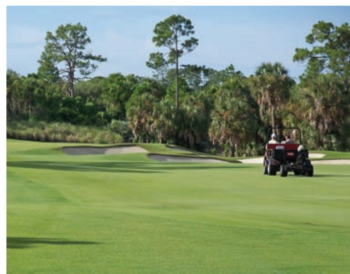
During mapping, a truckster pulls the remote sensing device as it takes soil moisture readings about every 10 feet (3 meters). Mapping an average fairway takes about 30 to 45 minutes. Photo by R. Carrow
