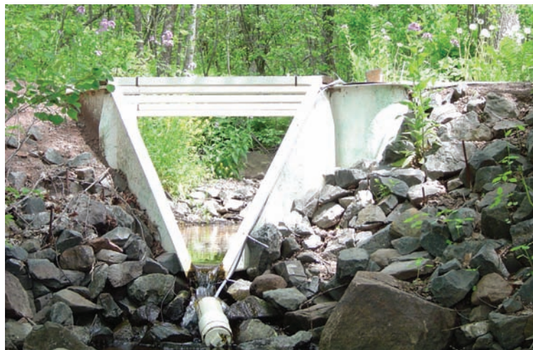
A bubbler flow meter was used to measure the depth of streams flowing through the golf course and into Lake Superior.
