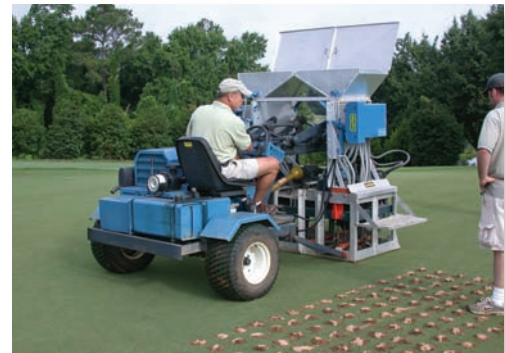
A drill-and-fill method was used to incorporate amendments into the putting green.
