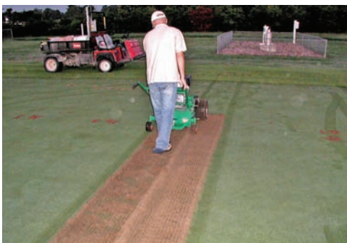
The Graden GS04 verticutter is capable of cutting channels through the surface organic layer of putting green root zones.
