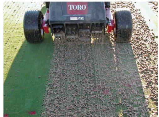
This greens aerator has been retrofitted with tine adapters allowing for a tine spacing of 1.25 x 1.5 inches. Photos by J. Landreth
