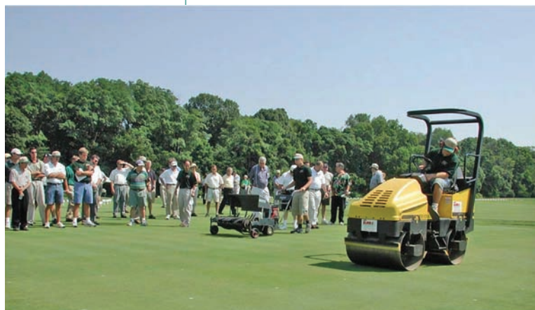
Compaction was simulated by making passes on the turf plots with a 952-pound, water-filled turf roller.
