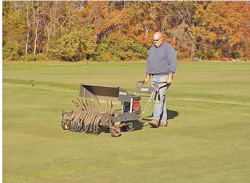
A wear simulator constructed from a modified walk-behind power broom was used to apply wear to putting green and fairway trials. Photos by J. Murphy
